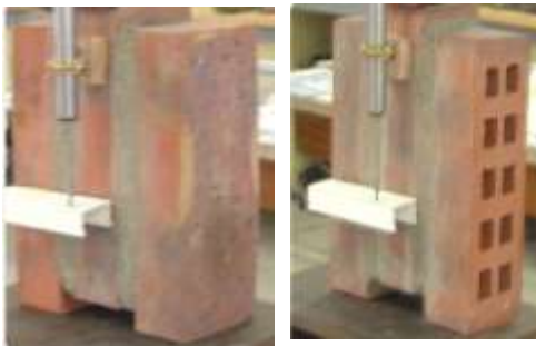
Shear test on hollow brick triplets [10]
