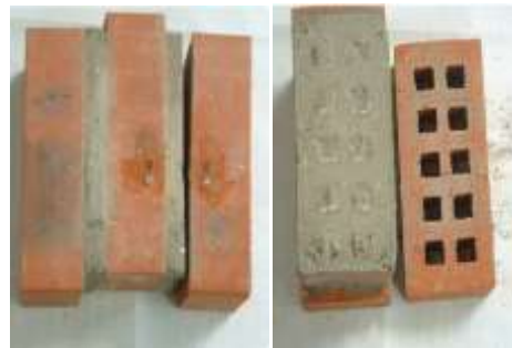
Strain due to shear test on the triplets [10,11]
